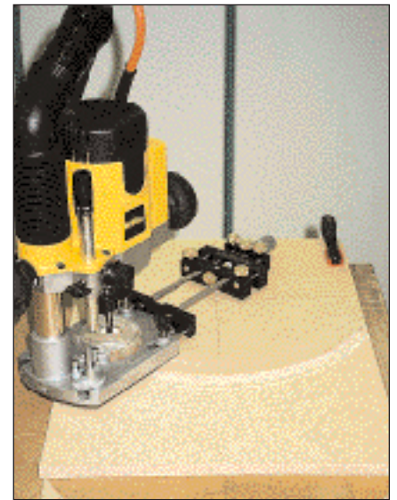
Cutting the inner radius with the Circle Jig
